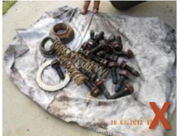
Examples of metal left inside a box that would have damaged the mulcher if un-detected
